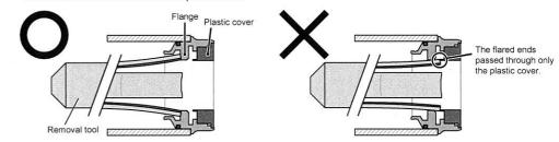
(2) Make sure that the flared ends engaged the flange, and then use a hammer to strike the tool head and taking out the right cup
