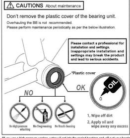
\*If you use a high pressure washer, water will get into the sealed bearings and will rust your bearings.
